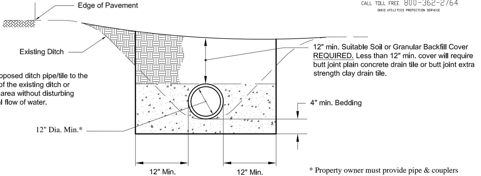
NOTE: Locate proposed ditch pipe/tile to the backside of the existing ditch or within the area without disturbing the natural flow of water.
