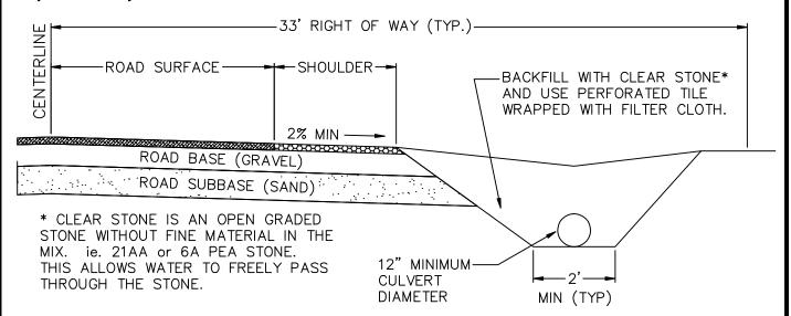
In both cases the swale ditch will require a positive outlet for the water it collects. This can be accomplished by draining into the open ditch beyond the enclosure or by placing a catch basin at the low point of the ditch enclosure. In no case should water be allowed to run along the edge of the road or over a driveway.
